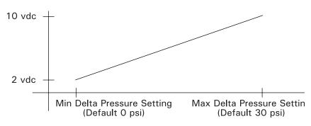
In this example, 2 vdc corresponds to 0 psi differential and 10 vdc corresponds to 30 psi differential. The min value of 0 psi, and the max value of 30 psi are individually adjustable via the service tool.
